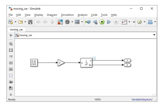
Simulating this model integrates a brief pulse twice to get a ramp and then displays the result in a Scope window. The input pulse represents a press of the accelerator pedal in a car, and the output ramp represents the increasing distance from the starting point.
