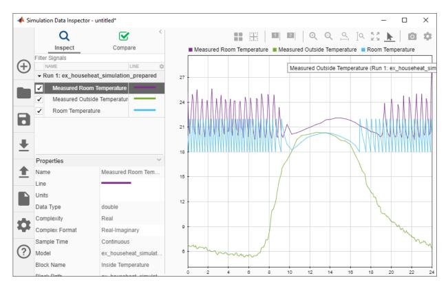
The top signal is the Measured Room Temperature. The middle signal is the Measured Outside Temperature. The bottom signal is the simulated Room Temperature.
