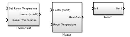
Notice the Thermostat subsystem now has a second input port. Each input port corresponds to an Inport block in the subsystem.
