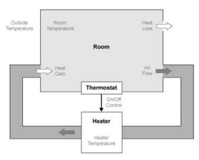
The model for this system includes three components: heater, thermostat, and room.
