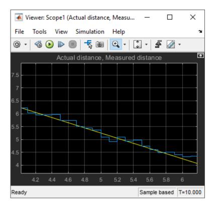
From the plot, you can see that the measurement can deviate from the actual value by as much as 0.3 meters. This information becomes useful when designing a safety feature, for example, a collision warning.
